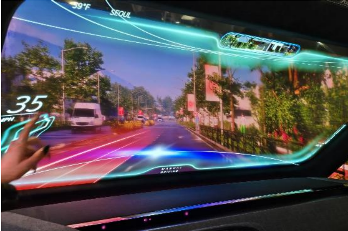
LG windshield display surface for real time information and mixed reality
